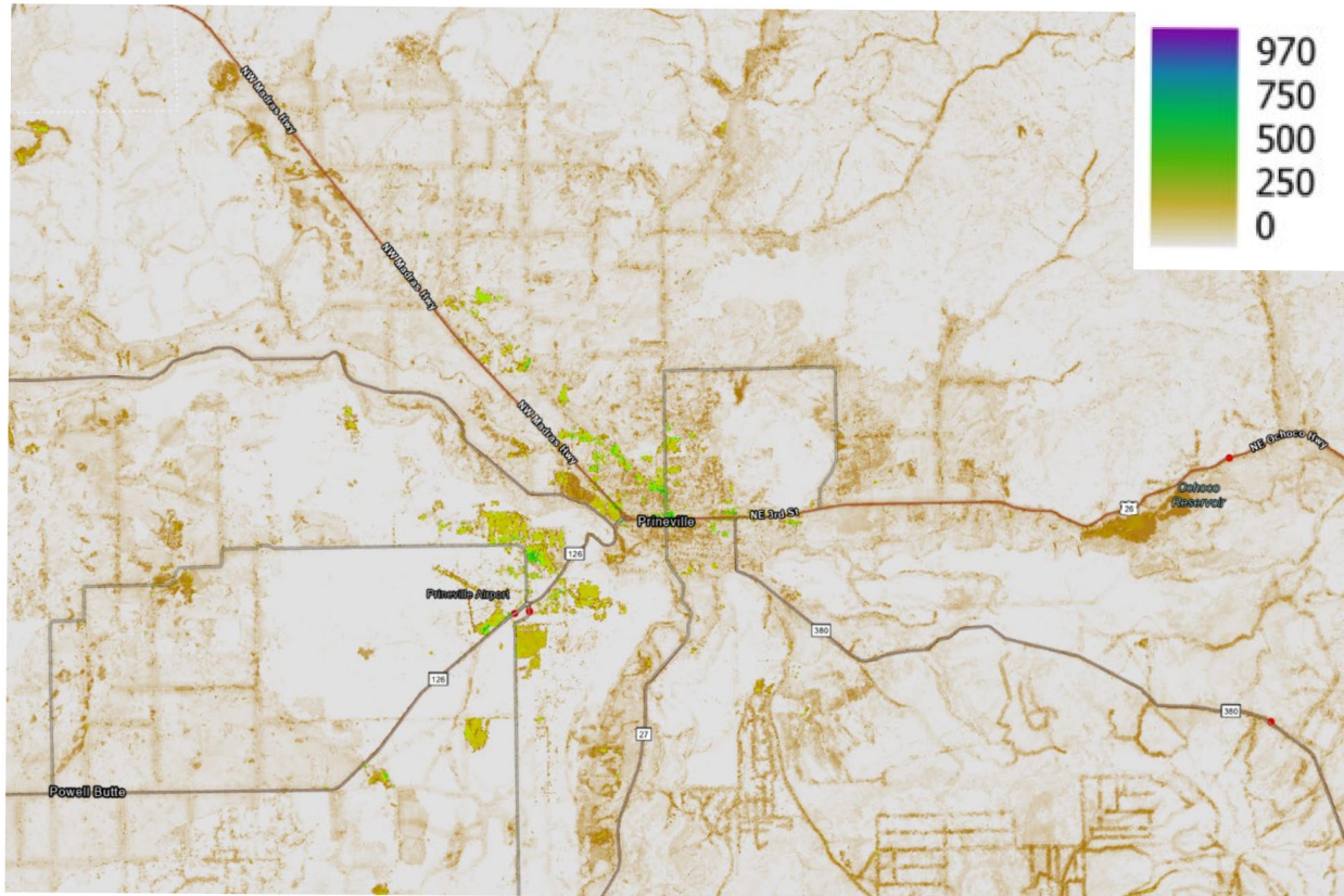
Figure 9. Ochoco Irrigation District estimated 'probability' surface from the random forest model. Raw model predictions have been multiplied by 1000.
